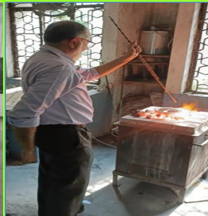
Crucible Furnace – Aluminium Melting in Foundry Shop
